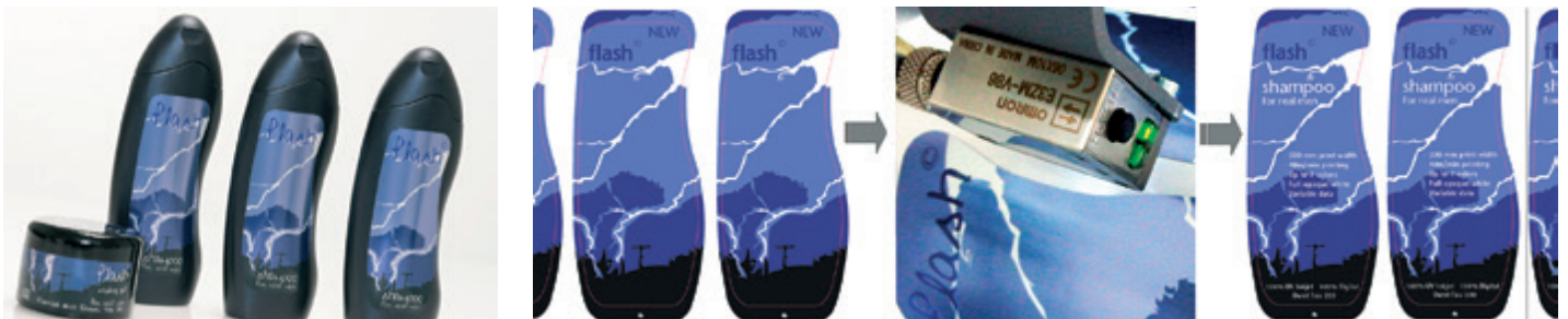
Late stage versioning of preprinted label jobs and printing on pre-die-cut label stock (blank labels)
